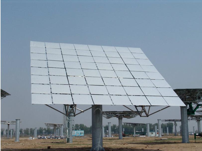
It is a compact unit drive that provide azimuth and zenith movement.
